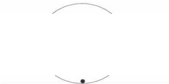
FIG. 1. The disc has mass M , radius R and is standing on a table where it rolls without slipping. The tiny dot at the bottom has no size and a mass m .
