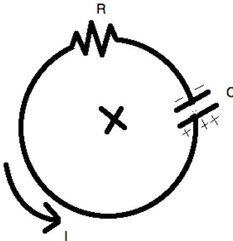
FIG. 1: The X indicates the direction of increasing magnetic flux, and thus by Lenz's law current must flow counterclockwise through the loop, depositing positive charge on the bottom end of the capacitor.
