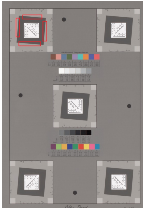
Figure 5. ROIs for the SFR/MTF computation (top left)
